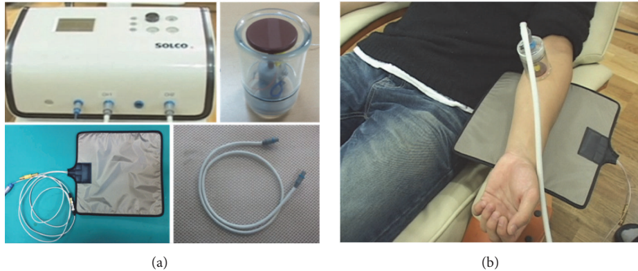
FIGURE 1: (a) Appearance and accessories of the PRF thermal stimulation device. From the left to right in a clock-wise direction: main body cup-shaped probe equipped with PRF radiation tip; connection cable; and electrode pad. (b) Example of the operation of the PRF thermal stimulation device.
