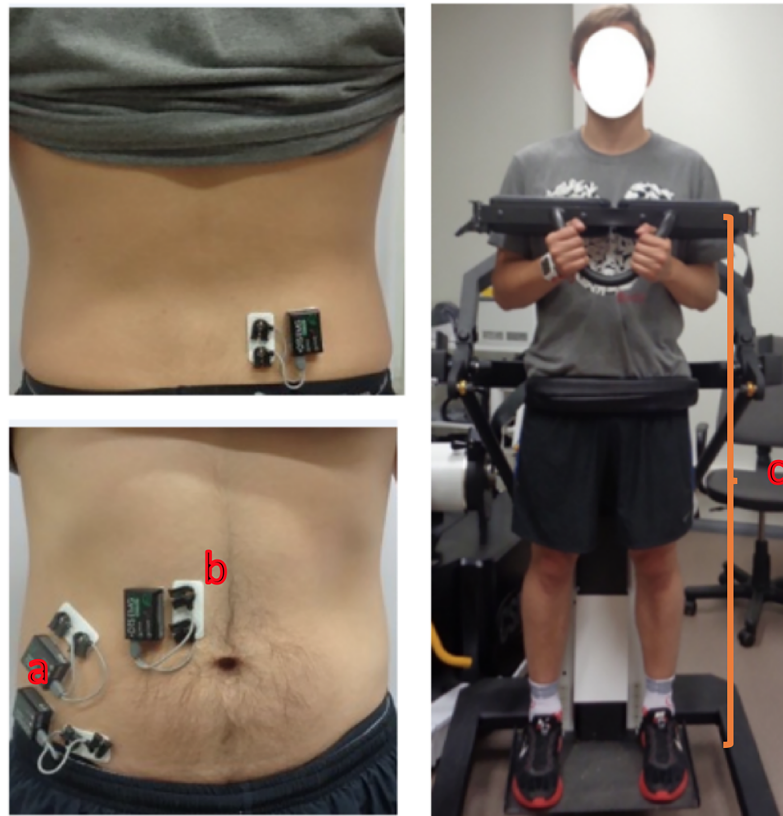
Fig 1. Preparation and the procedure of maximal isometric voluntary contraction with electromechanical dynamometer and surface electrodes. a) Direct transmission system (DTS) sensors, b) EMG electrodes c) electromechanical dynamometer.
