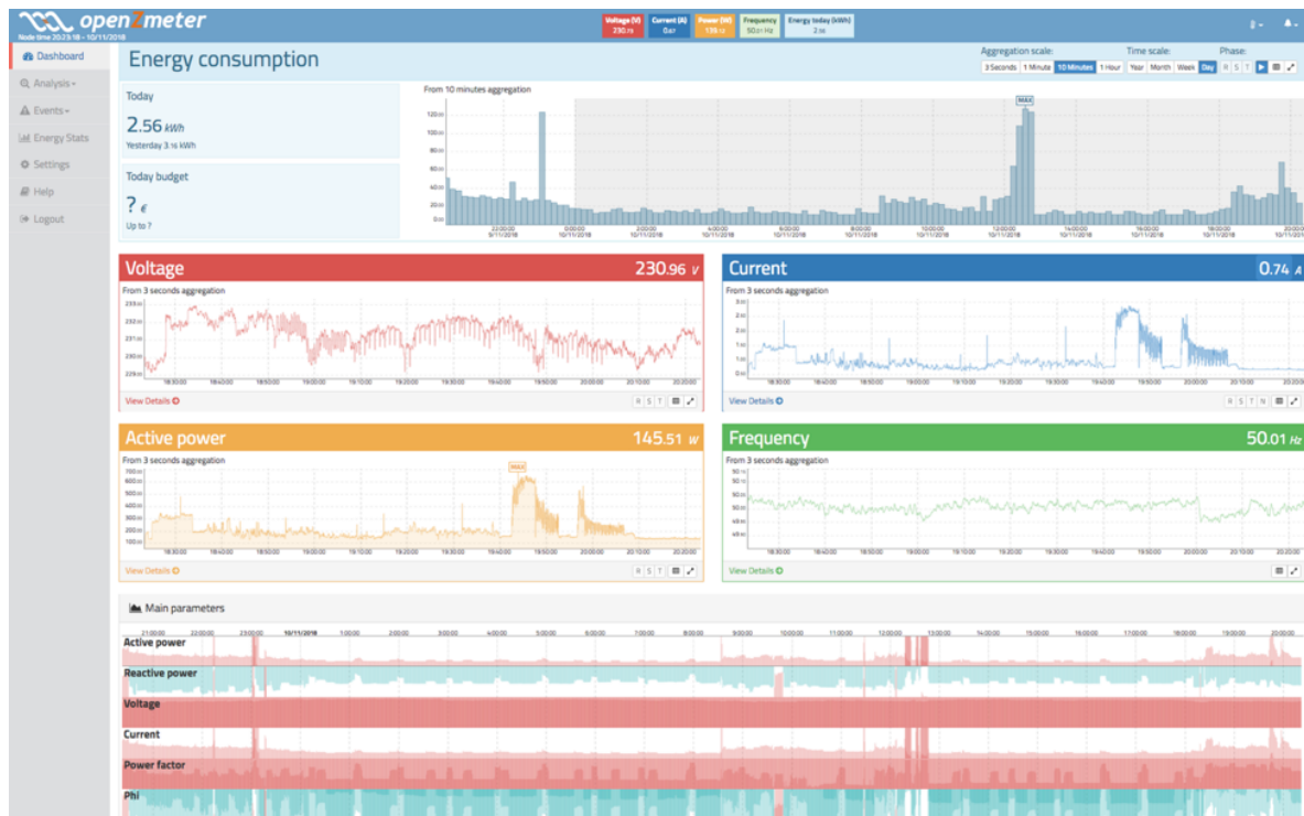
Figure 6. Dashboard of real-time power quality (PQ) monitoring and smart-metering software.
