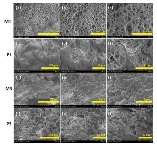
**Figure 4.** (**a**–**f**) SEM images of freeze-dried CS-g-PNIPAAm/PVA 80/20 (M1, P1) and (**g**–**l**) 75/25 (M3, P3). P1: CS-g-PNIPAAm/PVA *80/20* +PGT; M1: CS-g-PNIPAAm/PVA *80/20*; P3: CS-g-PNIPAAm/PVA *75/25* +PGT; M3: CS-g-PNIPAAm/PVA *75/25*.
