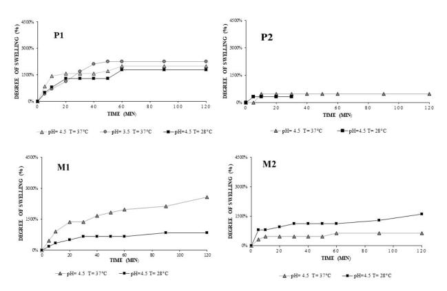
Figure 7. Swelling profiles at pH 4.5 and different temperatures for P1/M1 and P2/M2 hydrogels.
