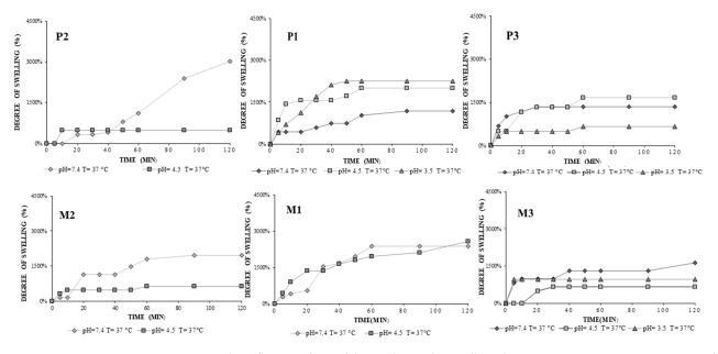
**Figure 6.** The influence of pH of the media on the swelling degree, at 37 °C. P1: CS-g-PNIPAAm/PVA 80/20 +PGT; M1: CS-g-PNIPAAm/PVA 80/20; P2: CS-g-PNIPAAm/PVA 95/5 +PGT; M2: CS-g-PNIPAAm/PVA 95/5; P3: CS-g-PNIPAAm/PVA 75/25 +PGT; M3: CS-g-PNIPAAm/PVA 75/25.
