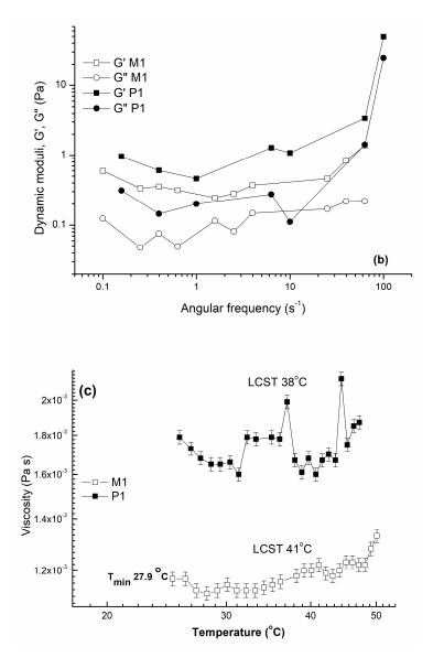
**Figure 3.** Rheological curves of CS-g-PNIPAAm/PVA 80/20 (M1) and CS-g-PNIPAAm/PVA 80/20-PGT (P1). (a) Viscosity dependency on the share rate and share stress–share rate curves; (b) Variation of dynamic moduli, storage G', and loss G" moduli with the angular frequency; (c) Temperature sweep curves.
