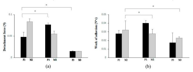
**Figure 10.** (a) Detachment force (N) at pH = 4.5. (b) Work of adhesion (N\*s) at pH = 4.5. Values were expressed as the mean (SD) from three independent experiments (n = 3). Each value represents the mean  $\pm$  standard error mean (n = 3). \* p < 0.05, One-way ANOVA Turkey HSD post hoc test.
