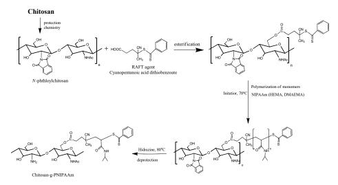
Figure 1. Synthesis approach of the CS-g-PNIPAAm via RAFT polymerization.
