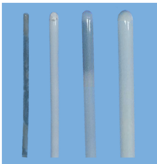
Figure 2 Locatable wires. There are four types of locatable wires with outer diameters of 0.75, 1.15, 1.45 and 1.95 mm (from left to right).
