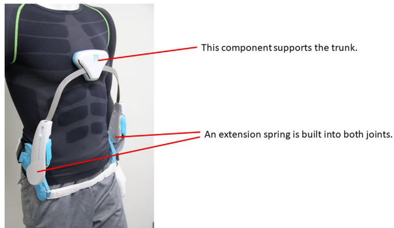
Fig. 1. Trunk Solution ® . The Trunk Solution ® has joints with springs and supports the trunk.
