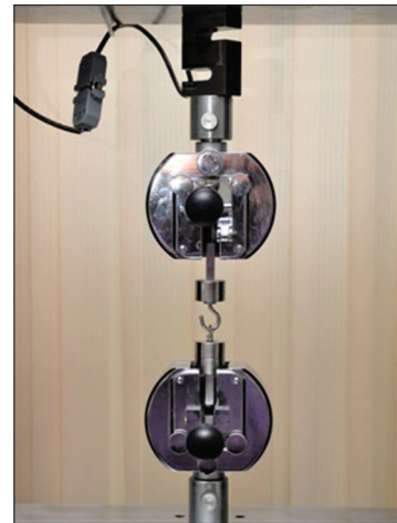
Figure 4: Crown pull test using universal testing machine
