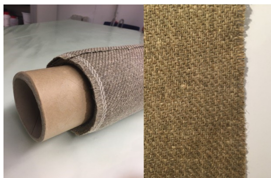
Figure 1. Flax fabric (area density of 550 \text{ g m}^{-2} , 7 yarn threads per cm in fabric warp and weft direction).
