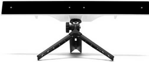
Fig. 9. Eye-tracker. Gazeport GP3 eye-tracker used in the experiment [6].
