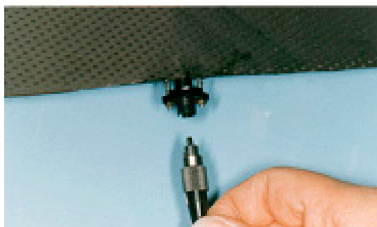
Figure 17. Egress optical fiber with connector.
