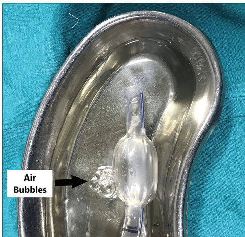
Figure 2: Air bubbles with lignocaine jelly under water demonstrating site of cuff leak
