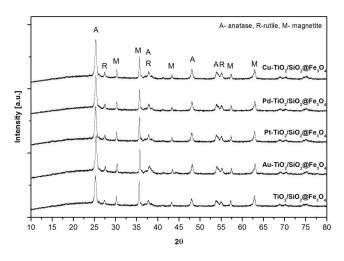
Figure 1. X-ray diffraction (XRD) patterns of Me-TiO<sub>2</sub>/SiO<sub>2</sub>@Fe<sub>3</sub>O<sub>4</sub> nanocomposites.
