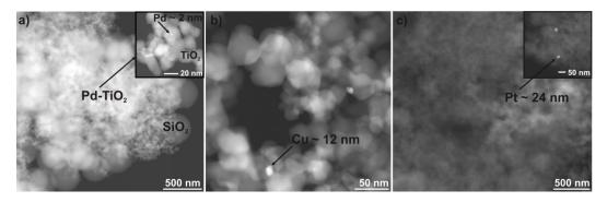
**Figure 3.** Dark-field scanning transmission (DF-STEM) microscopy images for (**a**) Pd-TiO<sub>2</sub>/SiO<sub>2</sub>@Fe<sub>3</sub>O<sub>4</sub>; (**b**) Cu-TiO<sub>2</sub>/SiO<sub>2</sub>@Fe<sub>3</sub>O<sub>4</sub> and (**c**) Pt-TiO<sub>2</sub>/SiO<sub>2</sub>@Fe<sub>3</sub>O<sub>4</sub> nanocomposites. Inserts for (**a**,**c**): magnification of metal nanoparticles deposited on TiO<sub>2</sub>.
