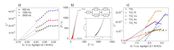
**Figure 4.** (a) Mott-Schottky plot of unmodified photocatalyst (space charge region capacitance calculated for 3 different frequencies); (b) Exemplary impedance spectrum and fitted data of unmodified  $TiO_2$  (recorded at 0 V vs. Ag/AgCl (0.1 M KCl). Insert: equivalent circuit used to model spectrum, and (c) comparison of Mott-Schottky plots recorded for  $TiO_2$ , Cu- $TiO_2$ , Pd- $TiO_2$ , Au- $TiO_2$ , and Pt- $TiO_2$  (capacitances calculated for 1000 Hz).
