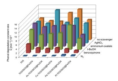
**Figure 8.** Photocatalytic degradation of phenol for Me-TiO<sub>2</sub>@SiO<sub>2</sub>/Fe<sub>3</sub>O<sub>4</sub> photocatalysts in the presence of  $e^-$ ,  $h^+$ ,  ${}^{\bullet}O_2^-$  and  ${}^{\bullet}OH$  scavengers and N<sub>2</sub> purging.
