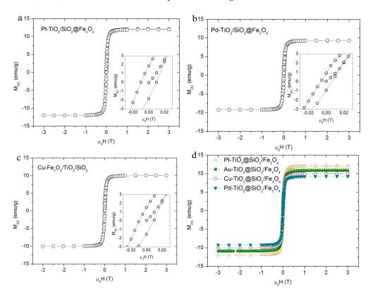
Figure 2. Magnetic hysteresis for (a)  $Pt-TiO_2/SiO_2@Fe_3O_4$ ; (b)  $Pd-TiO_2/SiO_2@Fe_3O_4$ ; (c)  $Cu-TiO_2/SiO_2@Fe_3O_4$ ; (d) all obtained  $Me-TiO_2/SiO_2@Fe_3O_4$  nanocomposites and magnification at hysteresis loop start point.
