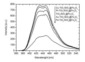
**Figure 7.** Fluorescence spectra changes observed during irradiation of Me-TiO<sub>2</sub>/SiO<sub>2</sub>@Fe<sub>3</sub>O<sub>4</sub> photocatalysts under UV-Vis irradiation.
