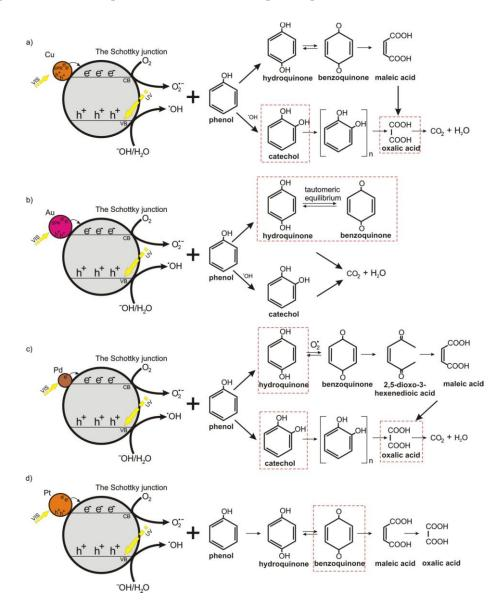
**Figure 9.** Schematic illustration of the phenol photocatalytic degradation mechanism for magnetic photocatalysts modified with: (**a**) copper; (**b**) gold; (**c**) palladium and (**d**) platinum nanoparticles.
