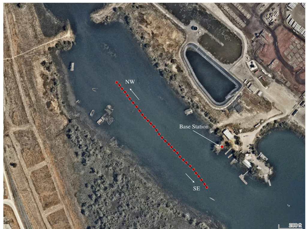
Fig 7. Satellite image showing a typical trial path. The single red dot on the shore is the location of the DGPS base station. The mean latitude and longitude are 38.566435° and -121.556365°, respectively.
