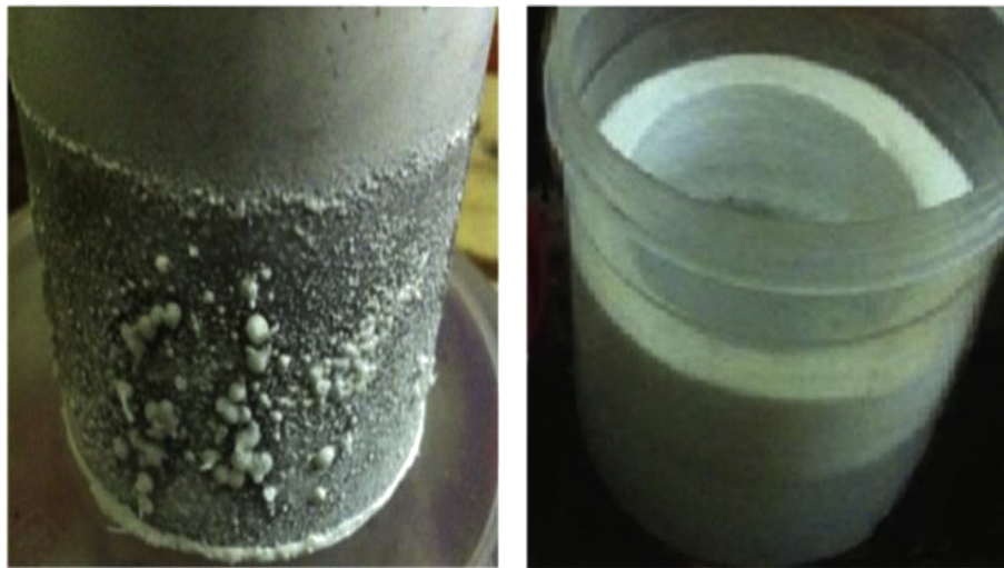
Figure 5. The aerated foams formed and salts transportation into the cathode surfaces during the treatment of 113400 mg TDS/L, 65623 mg TSS/L, and the ions of 477 mg HCO 3 /L, 102000 mg Cl/L and 5600 mg Ca/L real saline oily wastewater (reaction time = 25 min).
