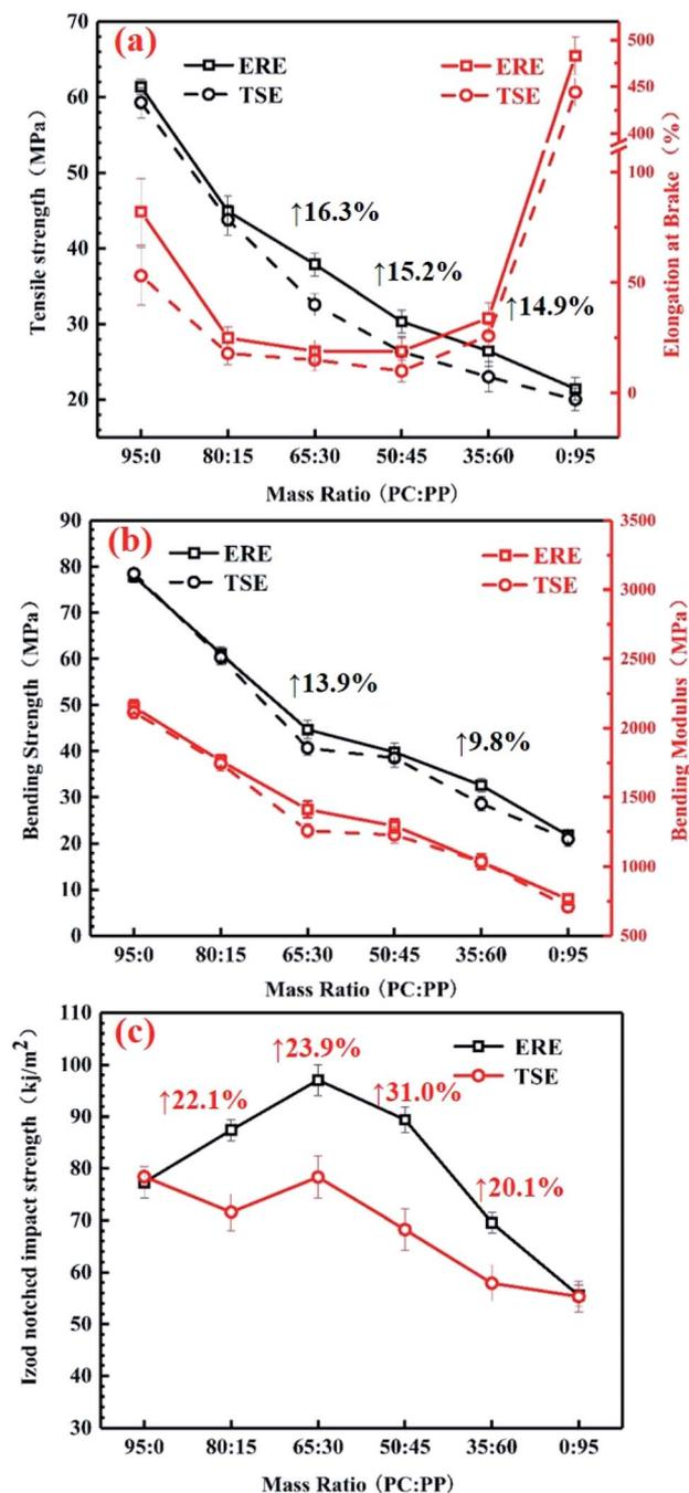
Fig. 6 Curves of mechanical properties versus mass ratio for PC/PP alloys by ERE and TSE (a) tensile strength and elongation (b) bending strength and modulus (c) notch Izod impact strength.
