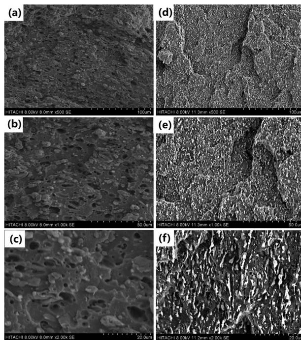
Fig. 7 SEM micrographs of injection moulded samples of PC/PP alloys (50 : 45) prepared by ERE and TSE. (a)  $\times 500$ -TSE (b)  $\times 1000$ -TSE (c)  $\times 2000$ -TSE (d)  $\times 500$ -ERE (e)  $\times 1000$ -ERE (f)  $\times 2000$ -ERE.
