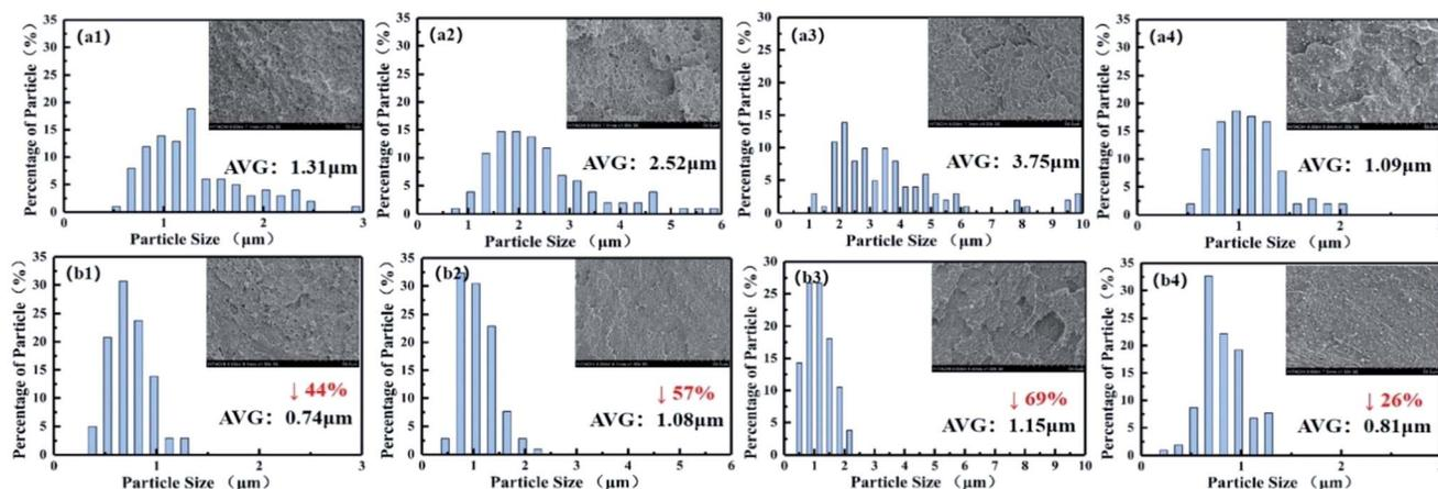
Fig. 5 SEM micrographs of extruded strips prepared by ERE and TSE and the statistical charts of the particle size of the dispersed phase. (a1) TSE-80 : 15 (a2) TSE-65 : 30 (a3) TSE-50 : 45 (a4) TSE-35 : 60 (b1) ERE-80 : 15 (b2) ERE-65 : 30 (b3) ERE-50 : 45 (b4) ERE-35 : 60.
