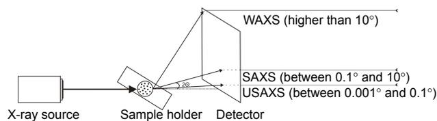
**Figure 2** Schematic mechanism of X-ray incidence into the sample and the classified scattering regimes (WAXS, SAXS, and USAXS), indicating the scattering angle explored by each one (WAXS:  $>10^\circ$ ; SAXS: between  $0.1^\circ$  and  $10^\circ$ ; USAXS: between  $0.001^\circ$  and  $0.1^\circ$ ).
