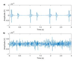
**Figure 1.** Comparison between (**a**) a good-quality signal (SNR = 31 dB) and (**b**) a poor-quality signal (SNR = 4 dB). The extraction of valve timing and even the SNR computation is evidently questionable in case (**b**).
