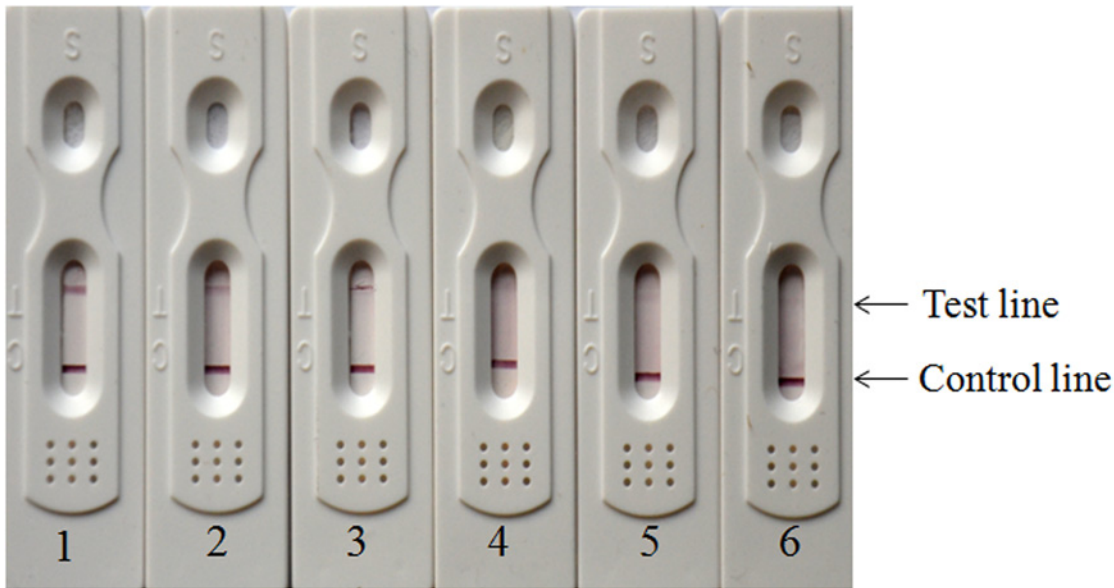
Fig 5. Sensitivity of colloidal gold immunochromatographic strips for detecting R. anatipestifer strain WJ4. 1–6, WJ4 at 10^8 , 10^7 , 10^6 , 10^5 , 10^4 , 10^3 CFU/strip respectively.
