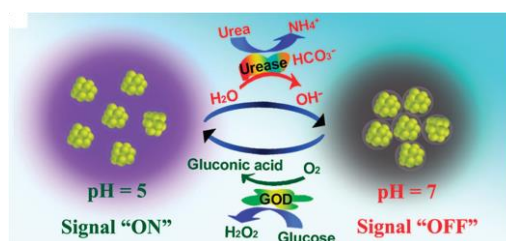
Figure 14. Schematic of the mechanism of the sensor for urea and glucose detection. Reproduced from Reference [114] with the permission of Nature Publishing Group.
