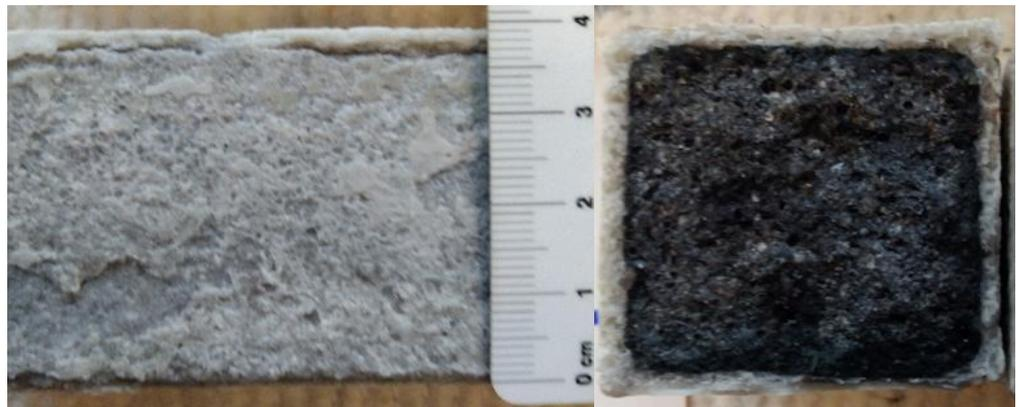
**Figure 15.** Surface degradation of mixture REF 2 deposited in XA3 solution.
