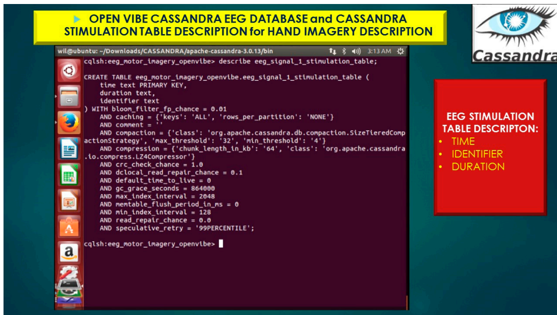
Figure 20. OpenVibe EEG Sensor Array stored in Cassandra NoSQL KEYSACE (database) with Simple_Strategy, Stimulation table, eeg_signal_1_stimulation_table importing eeg brain signal data (e.g., time, identifier, duration).
