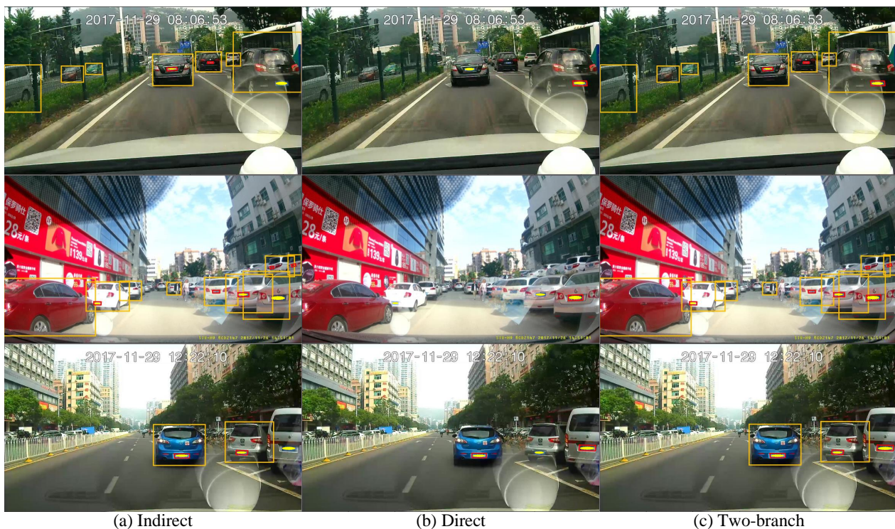
Figure 9. Detection results. The orange rectangle represents the horizontal bounding box of the vehicle. The red quadrangle indicates the quadrilateral bounding box of the license plate. Our method merges the detection results of the indirect and direct detection branches. All the recognizable license plates are manually covered with a yellow ellipsoid to protect privacy.
