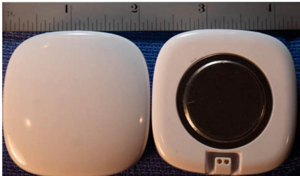
Figure 1 Image of heating units used in the study. The left image shows the side of unit that faces away from the skin. The right image shows the metal heating plate that is one inch in diameter. The heating plate rests on the skin over the area of pain and is held in place by an EKG-like sticker. In this study each subject received two heating units, one unit placed on the left paravertebral muscle at the L4/5 level and one on the right paravertebral muscle at the same level.
