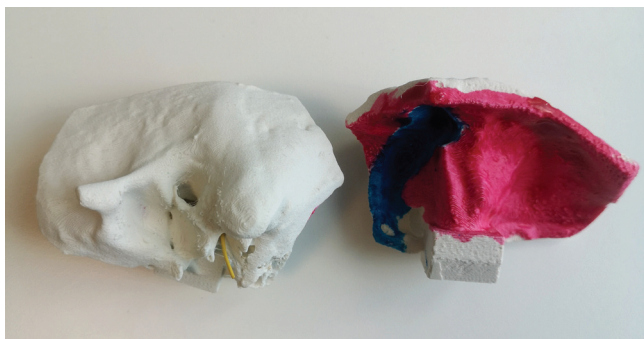
Figure 2. Views of the 3D-printed model. Left: frontal view. A yellow wire represents the facial nerve. Right: posterior view. The pink silicone layer represents the dura and the blue layer, the sigmoid sinus.
