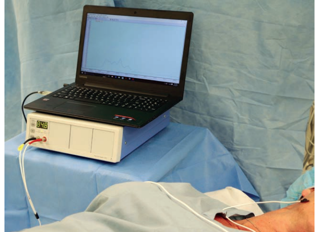
Fig. 2. A laptop computer is connected to the laser Doppler flowmeter using a data cord and software provided by the laser Doppler company. The laptop's desktop is configured using the free join.me app to become a teleconference host for screen sharing.
