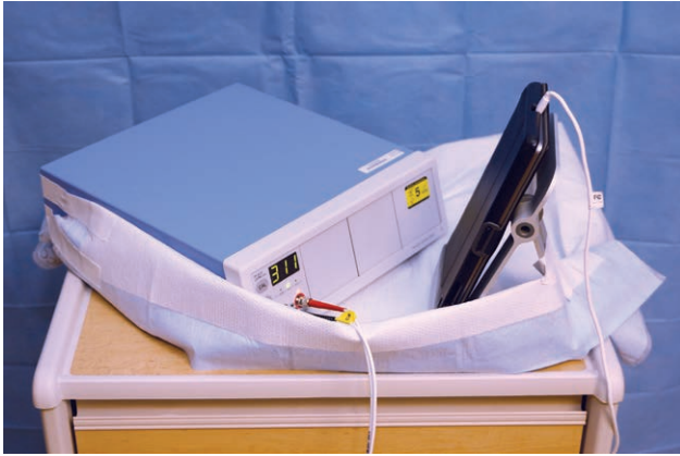
Fig. 1. The smart device (mini-iPad) with Wi-Fi capability is positioned next to the laser Doppler flowmeter with its camera capturing the digital readout. An underpad "cradles" the 2 devices to prevent dislodgement of the camera angle.
