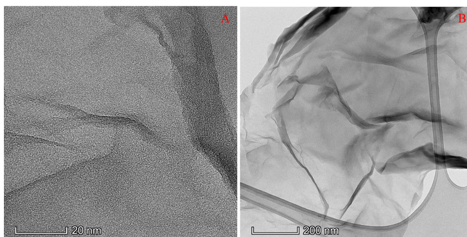
Figure 1 (A and B) TEM images of graphene oxide.
