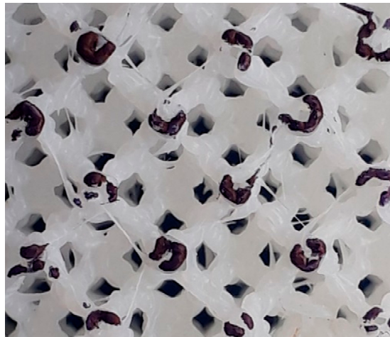
Figure 15. Cross-section of a CF lattice manufactured by ME. The colored surface highlights the deposited filament in a layer, with air gaps visible as the non-colored portion inside the darker contours.
