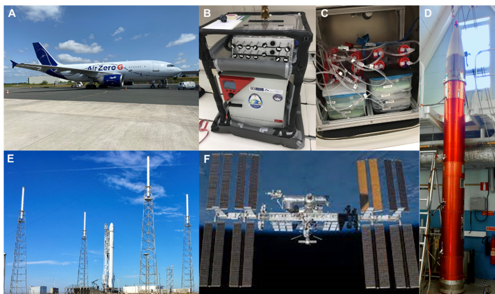
Figure 2. Real microgravity platforms. (A): 37th DLR Parabolic flight campaign, Airbus A310 Zero-g aircraft from the company Novespace in Paderborn, Lippstadt Airport, on 18 July 2021, (B): the PFC flight rack with an incubator and (C): open door of the incubator and boxes containing the cell culture flasks with DU-145 PCC. (D): Payload of a TEXUS-type sounding rocket (SSC, ESRANGE, Kiruna, Sweden; (E): SpaceX CRS-8 rocket on the launch pad, Kennedy Space Center (KFC), FL, USA; (F): the International Space Station.
