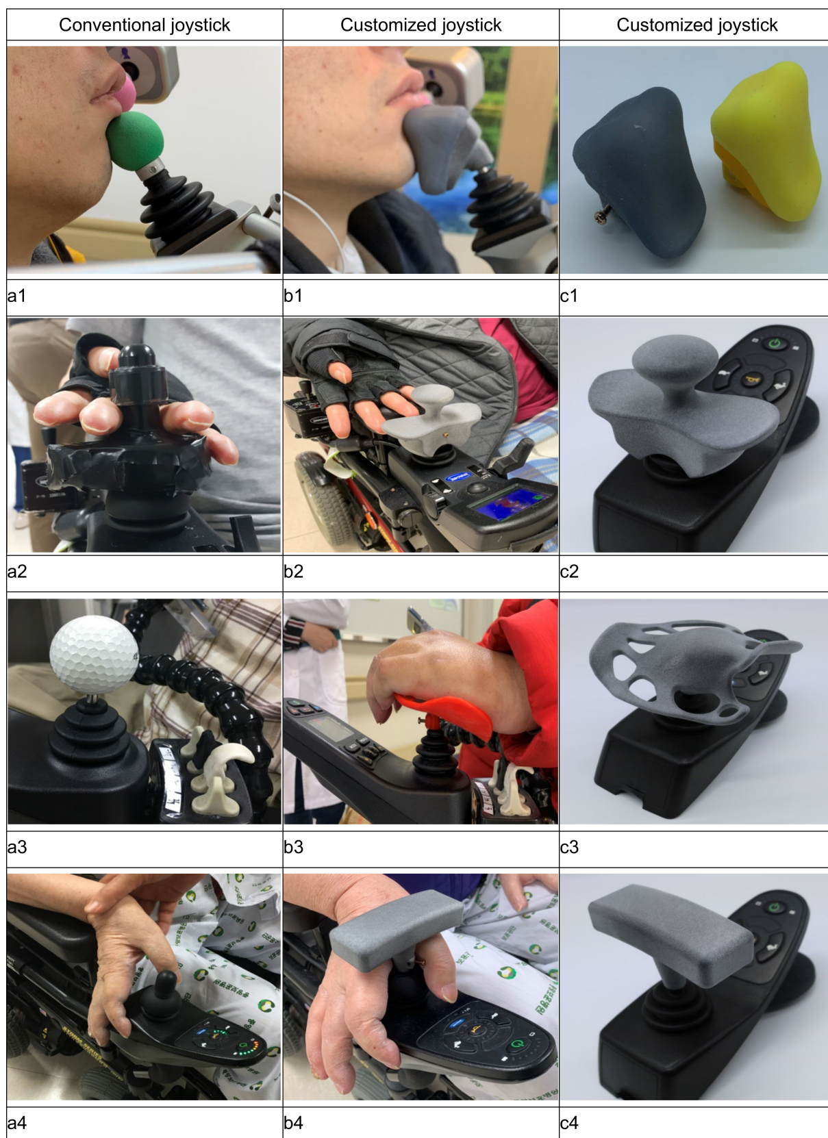
Figure 1. Joysticks employed in this study. (a) Conventional joystick. (b) Patient using the power wheelchair with a customized joystick. (c) Customized joystick.
