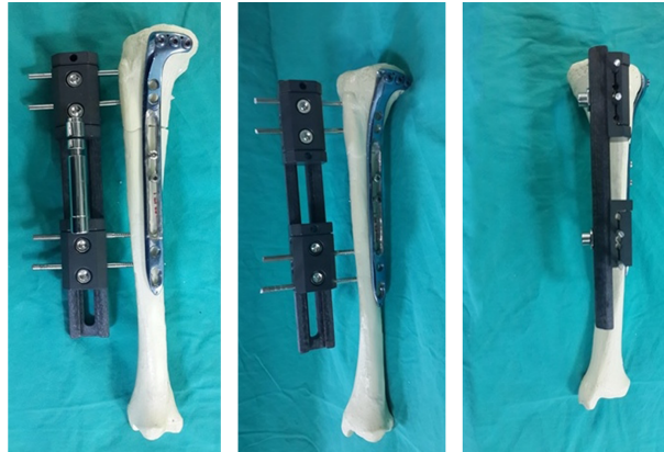
Figure 1. The External Fixator, Lengthening Plate, and Osteotomy Site are Shown Before Being Attached to a Tibial Composite Bone Model for Bone Lengthening
