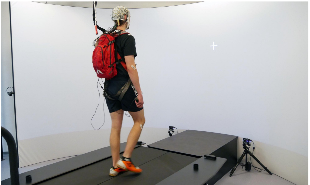
Fig 1. Participant performing the visual search task while walking on the GRAIL treadmill looking at the fixation cross. Stimuli were presented in the range from -40^{\circ} to +40^{\circ} degree visual angle and centered at eye level. In the perturbation blocks, the treadmill swayed randomly to the left or the right at the exact moment of stimulus presentation.
