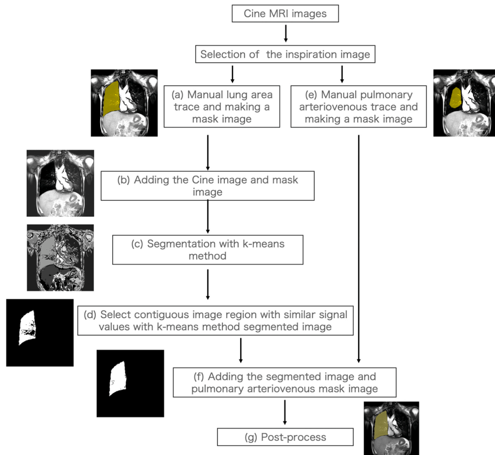
Fig. 1. Algorithm of the semi-automated lung segmentation program.
