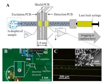
**Figure 1.** (**A**) Schematic illustration of capacitively coupled contactless conductivity detection ( $C^4D$ ) device on detecting bacterial concentration. (**B**) The printed-circuit-board (PCB) based electrodes. (**C**) Fluorescence-labeled *Escherichia coli* in capillary. (**D**) Scanning electron microscope (SEM) image of *E. coli*, the length of which on average is about 2  $\mu$ m.
