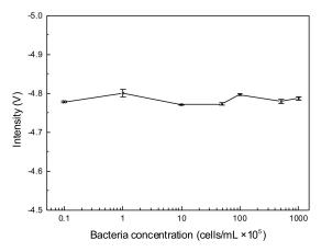
**Figure 3.** The  $C^4D$  response to the bacteria suspended in original phosphate-buffered saline (PBS) buffer with concentrations from  $10^4$  to  $10^8$  cells/mL. Error bars are standard deviations of four measurements.
