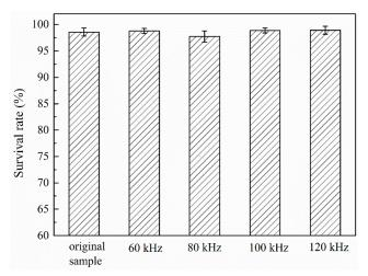
**Figure 2.** Influence on bacteria viability due to C<sup>4</sup>D detection by analyzing the ratio of live to dead cells. The recovered bacteria were labeled with Propidium Iodide (PI) and analyzed by flow cytometry (FCM). Error bars are standard deviations of four measurements.
