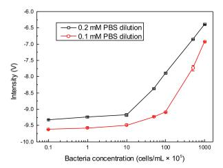
**Figure 5.** The C<sup>4</sup>D response to the bacteria suspended in 0.2 mM PBS dilution and 0.1 mM PBS dilution with the different concentrations of  $10^4$ – $10^8$  cells/mL. Error bars are standard deviations of four measurements.
