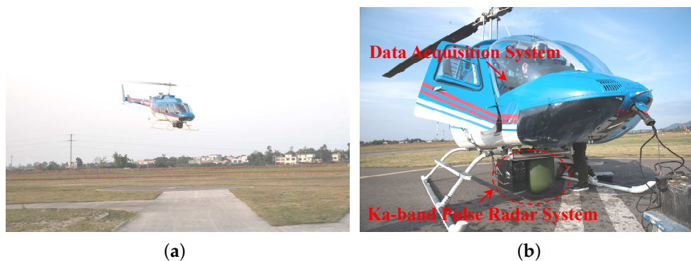
Figure 13. Experimental test platform: (a) Overview of the helicopter; (b) Onboard radar system.
