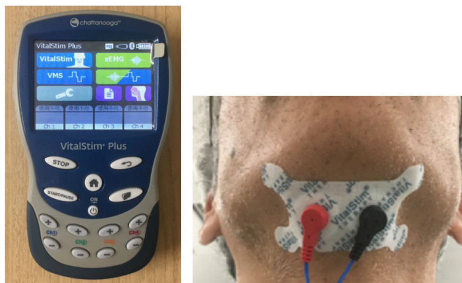
Figure 6. Neuromuscular electrical stimulation system (VitalStim ® Plus). The electrodes were attached to the submental area.
