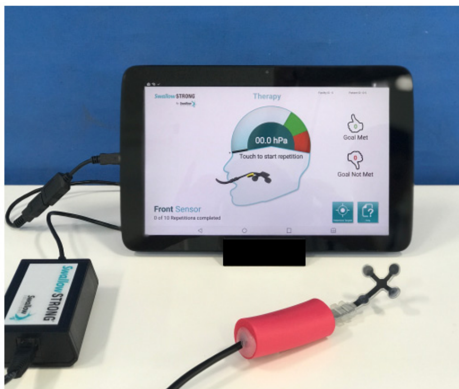
Figure 4. The Swallow STRengthening OropharyNGeal (Swallow STRONG). The device consists of custom-molded mouthpiece measuring tongue pressure and the tablet providing visual feedback.
