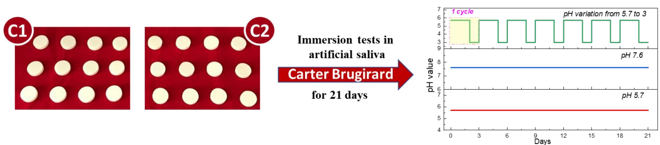
Figure 1. Images of the experimental samples (C1—Trinia TM and C2—TriLor) and pH value of the artificial saliva.
