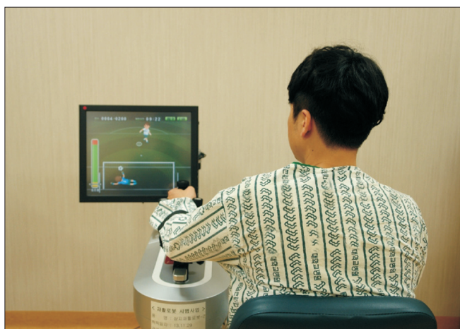
Fig. 1. Neuro-X system, an upper limb rehabilitation robot, consisted of a monitor and upper limb exercise equipment. The subject's posture was deviated at the right side from the robot.
