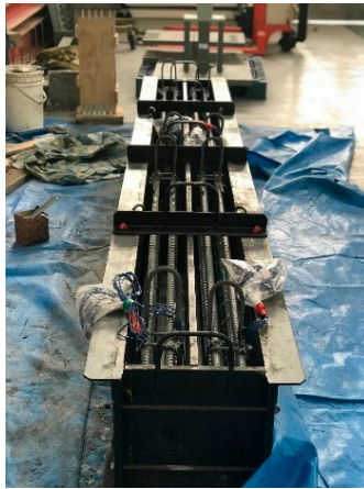
(a) Reinforcement cage of the UHPC beams
