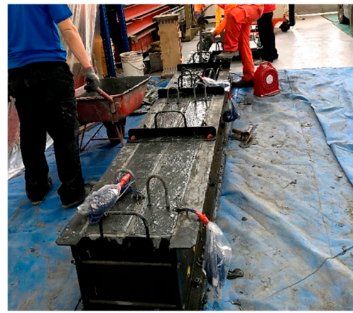
(b) Fabrication of the UHPC beams
