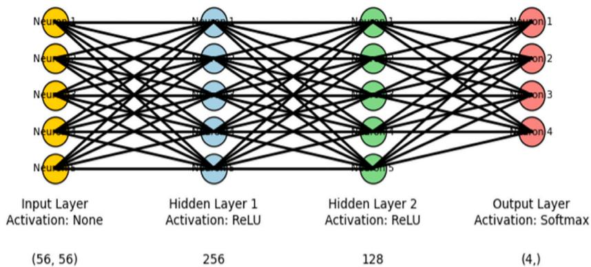
Fig. 2. Modified DNN Architecture for Motor Imagery BCI–Dataset2b with specified dimensions (MXN = 56X56).
