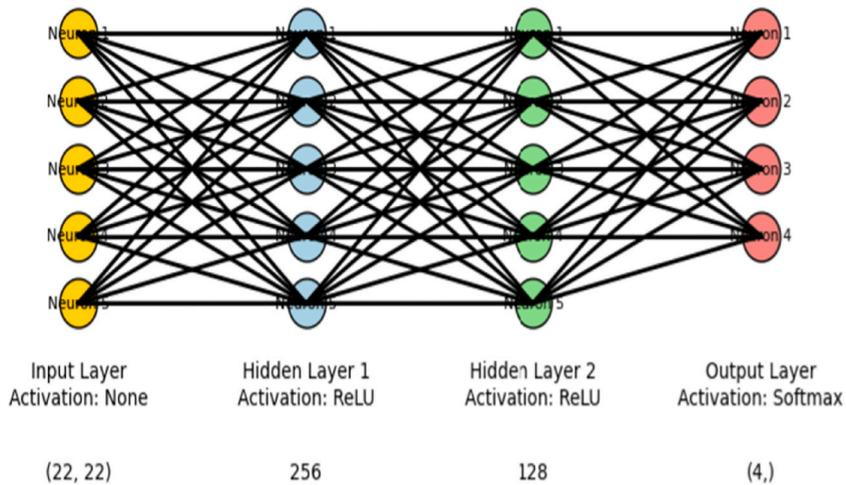
Fig. 1. Modified DNN Architecture for Motor Imagery BCI –Dataset 2a with specified dimensions(MXN = 22X22).
