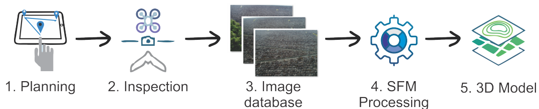
Figure 6. Aerial photogrammetry inspection process.
