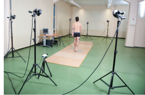
FIGURE 7: Recording and measurements of rotation kinematics parameters during gait using BTS Smart system.
