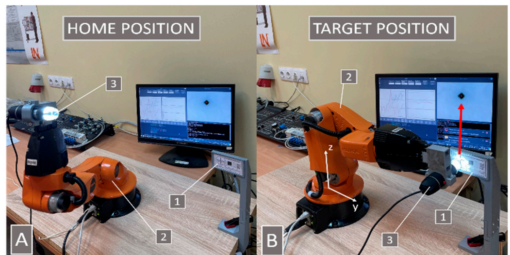
Figure 3. Robot “home” position (A) and the target position (B). The robot moved between these two positions during each cycle of the experiments. 1—target, 2—robot, and 3—microscope.
