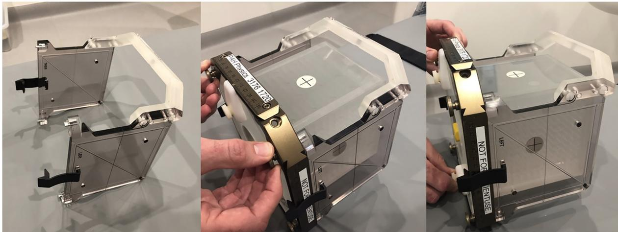
**Figure 1.** QUASAR™ GRID<sup>3D</sup> Image Distortion Phantom and MRI localizer box.
