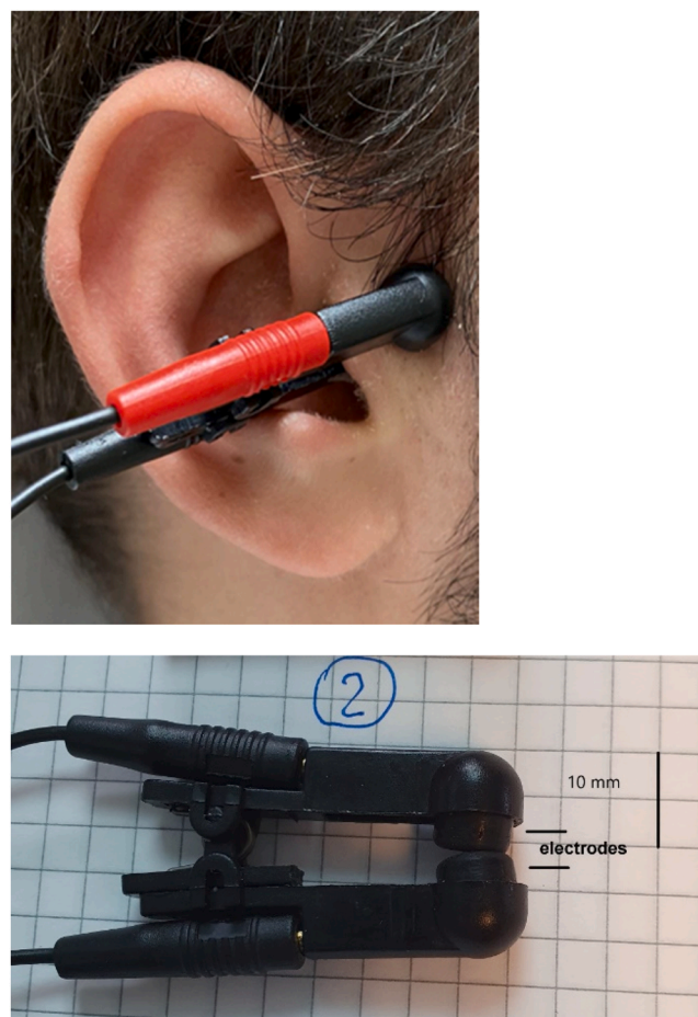
Fig. 1. We used two clip mounted conductive rubber electrodes attached to the inner skin surface of tragus/cavum conchae area, near the external auditory meatus, and outer tragus skin surface of the right ear. For better skin contact a conductive paste was applied and the clip was secured with adhesive tape.
