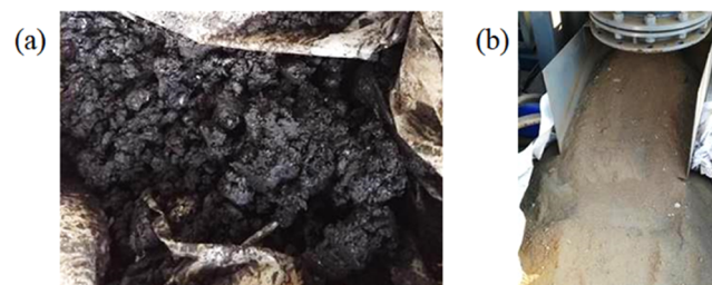
Figure 13. Oil-based cuttings (a) before and (b) after treatment.
