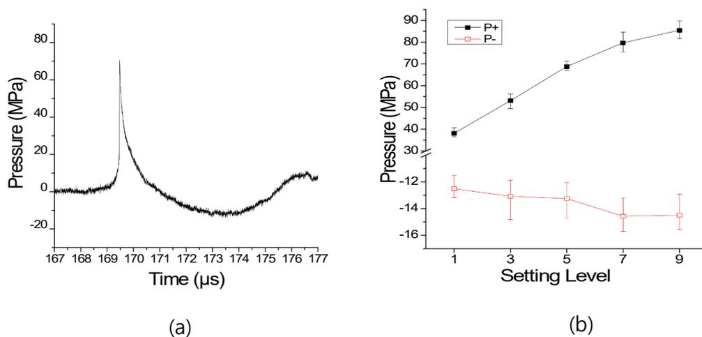
**Fig. 2.** (a) The typical shock pulse produced in water by the EM type shock wave generator (Rifle, HnT Medical System, Rep. Korea), measured at the focus using an optical hydrophone (FOPH200, RP Acoustic, Germany), and (b) peak pressures against output settings (N = 40).
