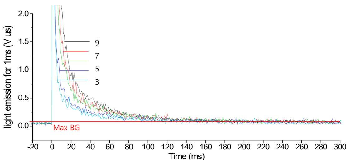
Fig. 7. Temporal history of the extent of the LE calculated every 1 ms in the luminol solution at the output settings of 1, 3, 5, 7 and 9. Note that the horizontal line represents MBGL.
