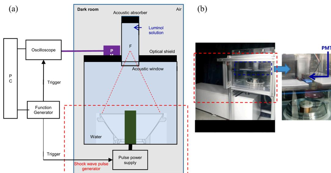
**Fig. 1.** Experimental setup: (a) Schematic functional diagram and (b) photograph. It consists of a shock pulse generator, PMT, a small acrylic resin structure, a digital oscilloscope, Function Generator, and PC.
