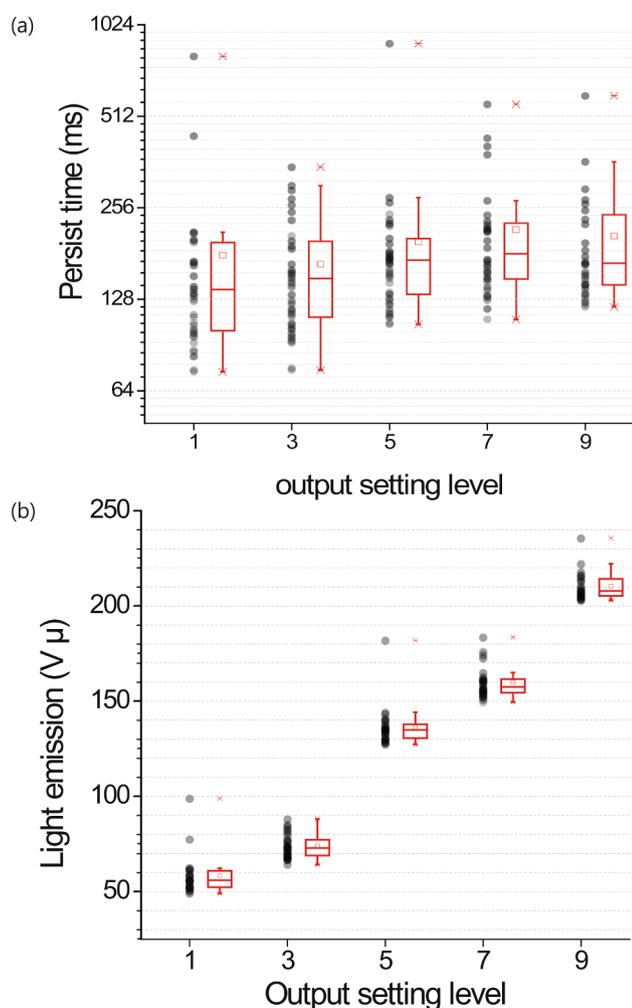
Fig. 8. (a) The time that OH\* FR is expected to persist, and (b) the extent of LE as the setting level increase, obtained from the 10 averaged temporal history of 1 ms LE from the luminol solution.
