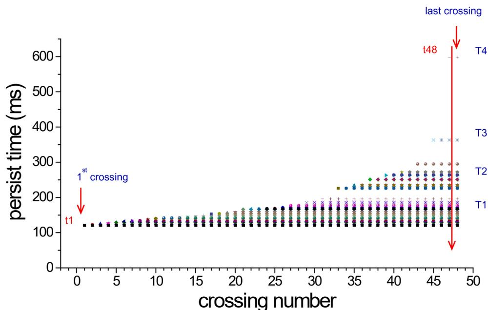
Fig. 6. Corresponding persist time from the 1st crossing ( $n = 1$ ) to the last crossing ( $n_{max}$ ).
