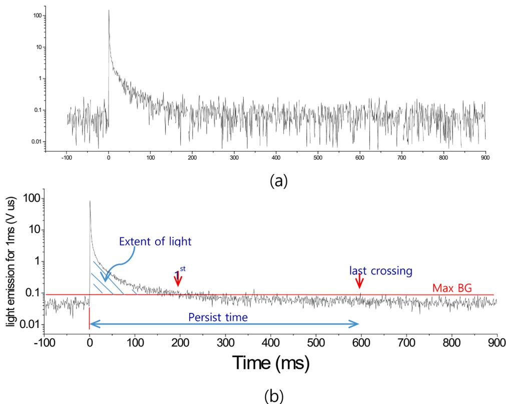
Fig. 5. Temporal history of the extent of LE measured in the luminol solution at the maximum output settings of 9. The vertical axis represents the quantity of light calculated by integrating the LE pulses above the dark noise level of 0.02 V for 1 ms: (a) single measurement, (b) average with 10 repeated records. Note that the persist time ranges from the 1st crossing to the last crossing of the signal to the max BG level ( $=0.1094$  V us).
