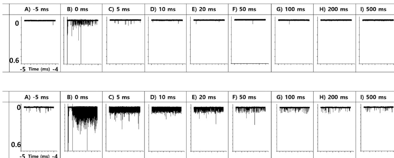
**Fig. 4.** The detailed LE signals recorded for 1 ms at the different time locations of A =  $-5$  ms, B =  $0$  ms, C =  $5$  ms, D =  $10$  ms, E =  $20$  ms, F =  $50$  ms, G =  $100$  ms, H =  $200$  ms, I =  $500$  ms at the sampling time of 10 GS, illustrating the temporal density of the LE pulses gradually decreasing with time: (a) water, and (b) the luminal solution.
