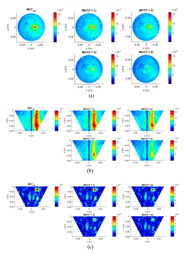
**Figure 6.** UWB images of the five phantoms demonstrating the correlation between intensity of the image  $I(\mathbf{r}_0, T)$  reconstructed via Equation (6) and the decreasing permittivity of the tumor imitate in (a) xy-slice, depth z = -2 cm and (b) in xz-slice, y = 0. The magnitude of the common DAS imaging (Equation (4)) is shown in (c). Color bar represents the intensity of the image in the arbitrary units.
