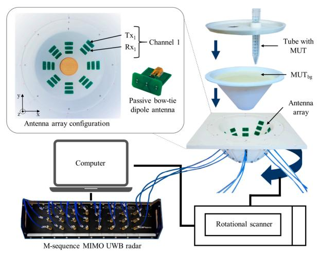
**Figure 3.** Measurement setup for preliminary investigations towards tissue temperature estimation. MIMO stands for multiple input multiple output, UWB for ultra-wideband and MUT for material under test, index in  $MUT_{bg}$  stands for background.
