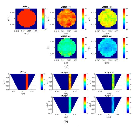
**Figure 7.** Distribution of the estimated relative permittivity  $\underline{\hat{\varepsilon}}_t(\mathbf{r}_0, \omega, T)$  at 2 GHz based on Equation (10) in the tumor area (a) in xy-slice, depth z = -2 cm and (b) in xz-slice, y = 0. Color bar represents the relative permittivity value.
