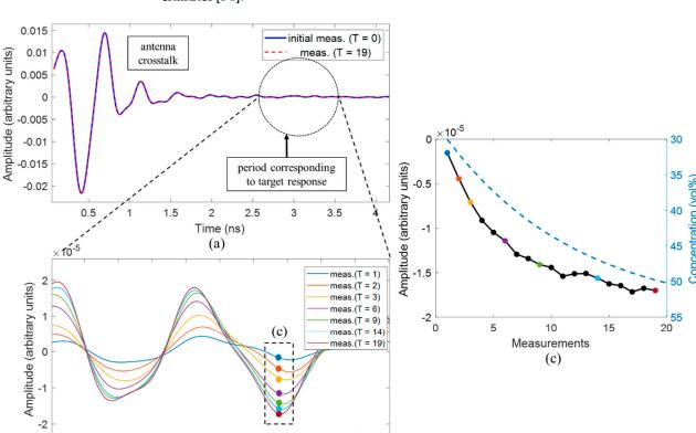
by antennas crosstalk removal by means of rotational average value subtraction of each channel [34].
