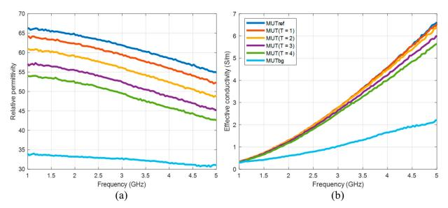
Figure 4. (a) Relative permittivity and (b) effective conductivity of MUTs as a function of frequency.
