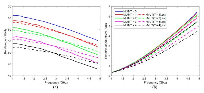
**Figure 9.** Estimated mean relative permittivity (**a**) and effective conductivity (**b**) in the 3D tumor area as function of frequency (dashed lines) and measured by means of dielectric spectroscopy (solid lines).
