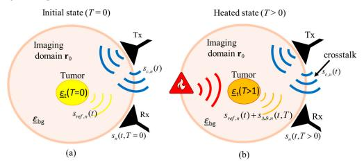
**Figure 2.** Schematic of the measurement scenario of temperature estimation during hyperthermia by means of UWB sensing (a) before start of treatment and (b) during treatment.
