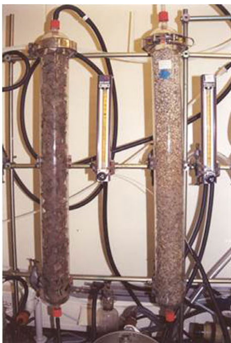
Fig. 2. An example of a laboratory-scale biofiltration system using C. psammophila as the biocatalyst for the elimination of toluene. The presence of the fungus can be observed by the darkening of polyurethane foam (left) and perlite (right) (Prenafeta-Boldú et al. , 2008). Image courtesy of Dr. Francesc X. Prenafeta-Boldú.
