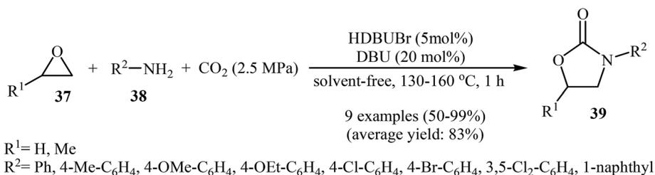
Scheme 19 DBU/HDBUBr-catalyzed three-component synthesis of 3-substituted-2-oxazolidinone **39**.
