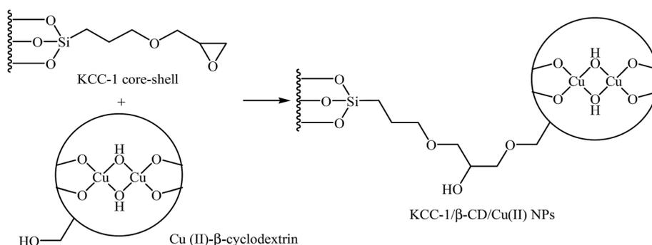
Scheme 23 Schematic illustrations of the synthetic route of KCC-1/β-CD/Cu(II) NPs.
