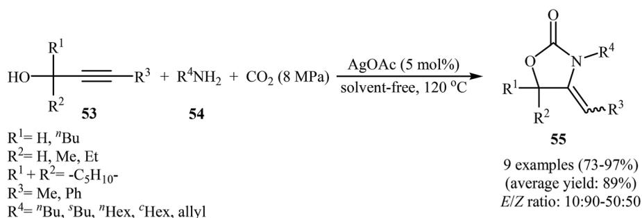
Scheme 26 Ag-catalyzed three-component coupling of propargylic alcohols **53**, amines **54**, and  $\text{CO}_2$  reported by Jiang and Zhao.
