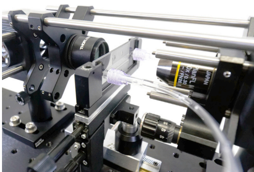
Figure 10. Slit flow shear chamber secured and positioned in the sample stage holder assembly Note: Objective lens assembly retracted out of the way for picture.
